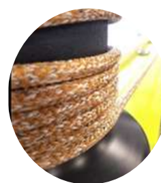
PBO Zylon + DYNEEMA cover tested at Soluzioni Tessili Rigging work bench
